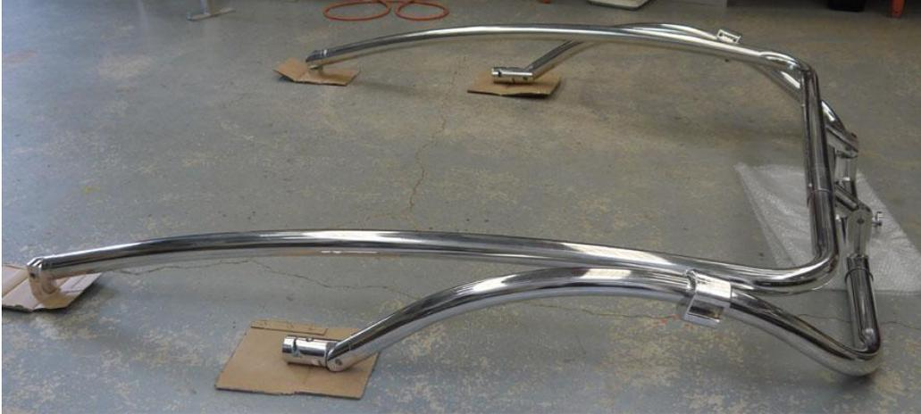
Only fold the tower down for storage, transport the tower in the upright position as this is when the tower is strongest and most stable.
